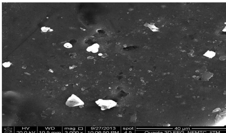
**Fig 3. SEM image of the formulation F3 before dissolution**
