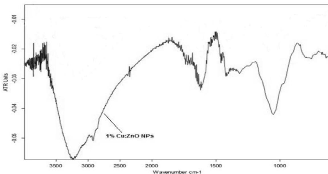
**Fig.4: FTIR Spectra of Cu:ZnO Nanoparticles**
