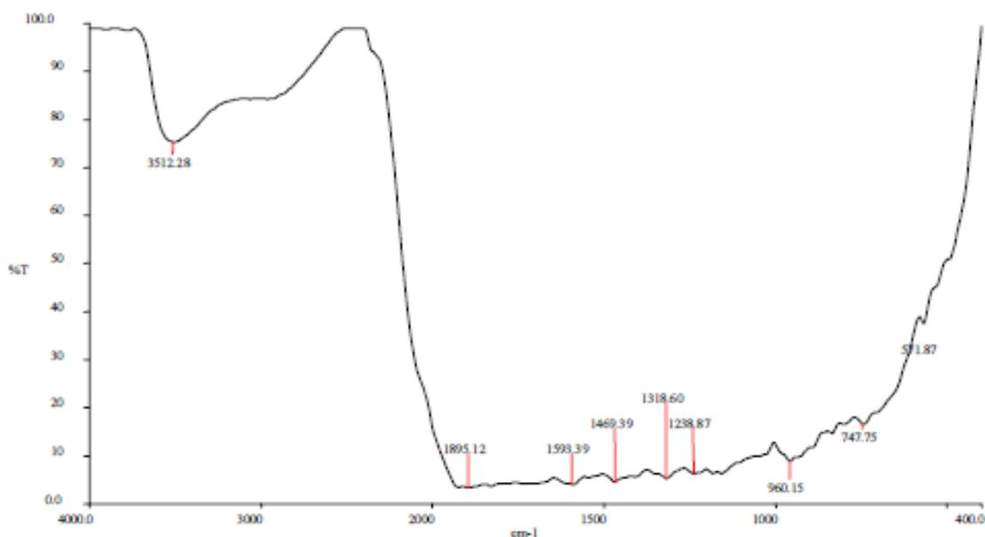
**Fig. 3: FTIR Spectra of ZnO Nanoparticles**
