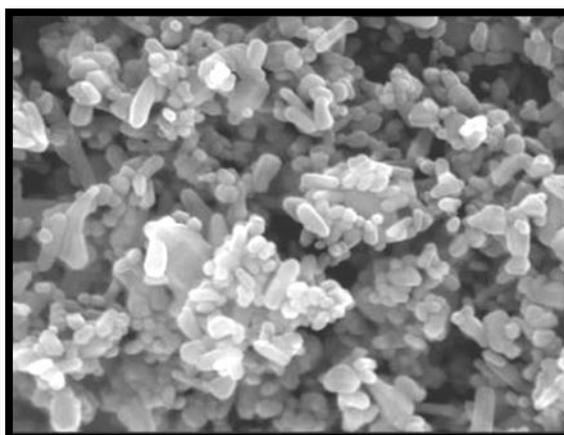
Fig. 2: SEM Image of Cu:ZnO Nanoparticles
