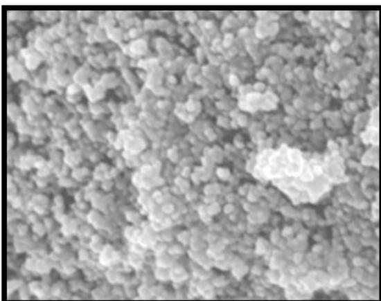
Fig. 1: SEM Image of ZnO Nanoparticles
