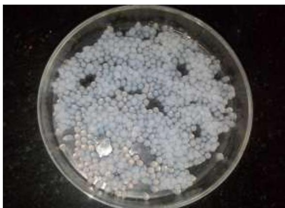
**Fig. 1: Drug loaded IPN Hydrogel beads in  $AlCl_3$  (cross linker) solution during Curing**
