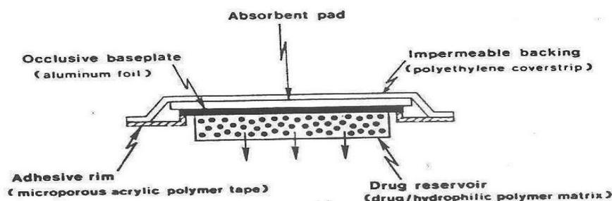
Figure 4: Matrix dispersion-type transdermal drug delivery system
