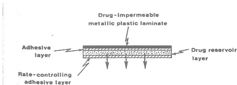
Figure 3: Adhesive diffusion-controlled transdermal drug delivery system.
