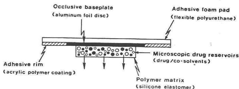
Figure 5: Micro reservoir-type transdermal drug delivery system<sup>[11]</sup>
