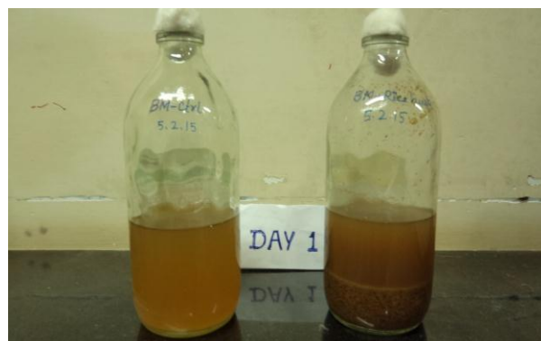
Solid State Fermentation in Basal Medium and Rice Husk Substrate in Basal Medium
