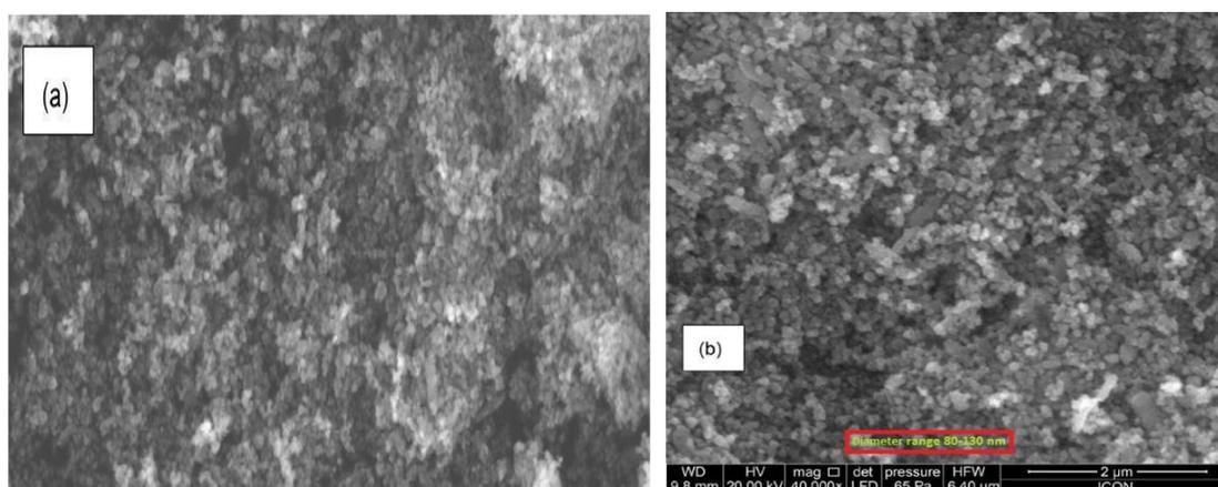
**Figure 2[a] & [b]:** SEM image of the synthesized zinc oxide nanoparticles.
