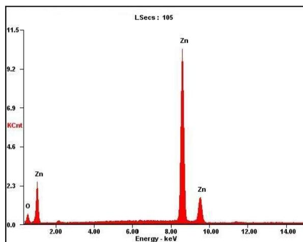
**Figure 3:** EDX spectrum of synthesized zinc oxide nanoparticles.
