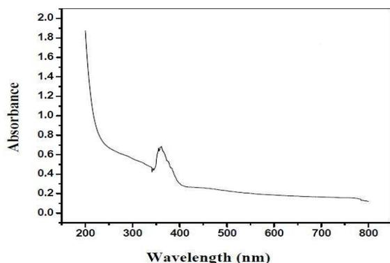
**Figure 1:** UV-Visible spectrum of synthesized ZnO-NPs.
