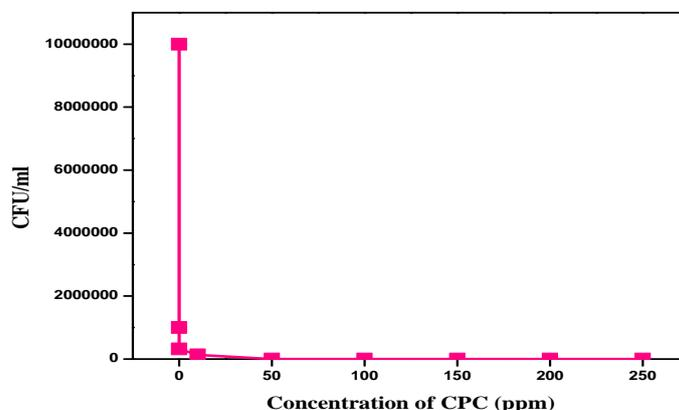
Fig.9 Biocidal Efficiency of CPC as a function of number of colony forming units in relating to concentration of biocide CPC
