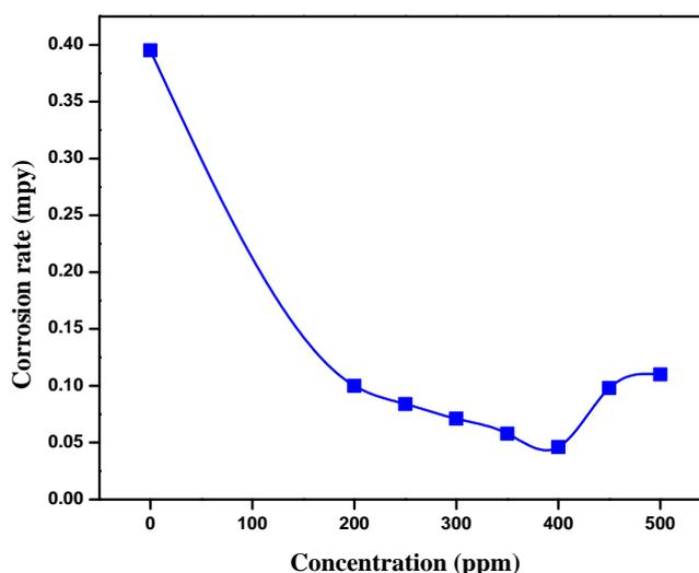
**Fig. 3: Plot of corrosion rate with various concentration of the inhibitor system 5MBTA+SPT.**
