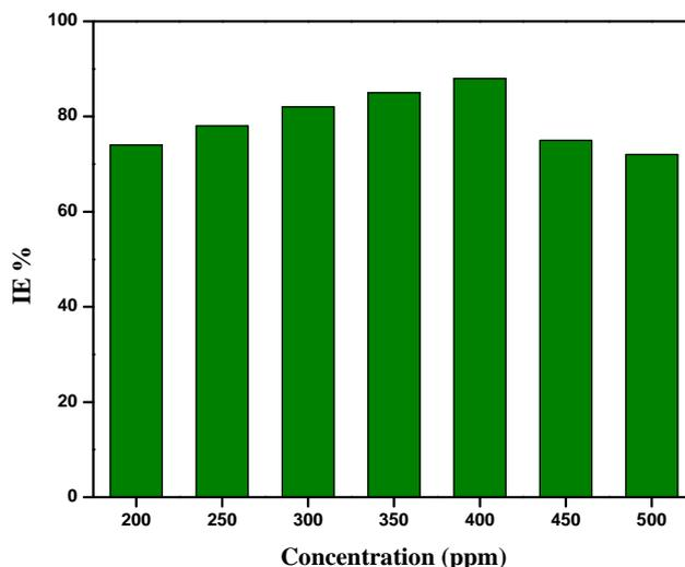
Fig.4 Plot of inhibition efficiency with various concentration of inhibitor 5MBTA+SPT.
