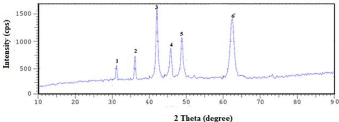
Fig. 6: XRD patterns of brass surface immersed in 3% NaCl.
