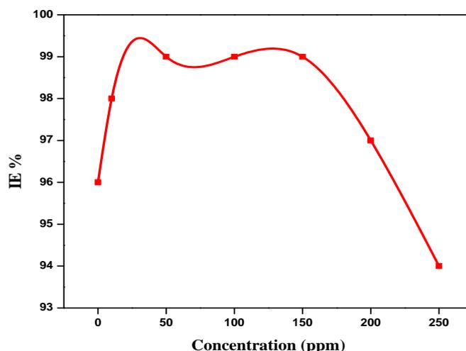
Fig.11 Effect of SDS on IE of 5MBTA+SPT.
