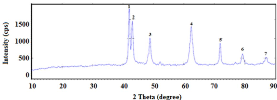
Fig. 7: XRD patterns of brass surface immersed in 3% NaCl containing 5MBTA+SPT.
