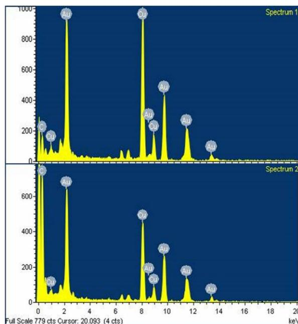
**Fig. 4: EDS of samples synthesized with incubated extract (spectrum 1) and boiled extract (spectrum 2).**
