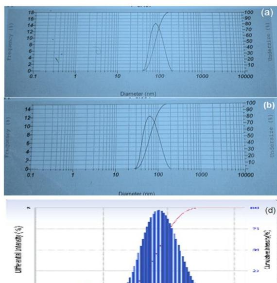
Fig. 7: Zeta Size distribution of synthesized gold nanoparticles with incubate (7-a), boiled extracts(7-b) and Size distribution by intensity(7-d).
