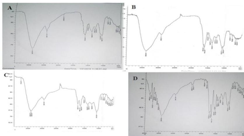
**Fig. 8: FTIR spectrums of seeds incubated extract(A), boiled extract (B) and synthesized gold nanoparticles with incubated extract(C), boiled extract (D).**
