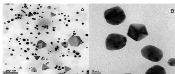
**Figure 5: TEM for samples synthesized with incubated extract (A) and boiled extract (B).**
