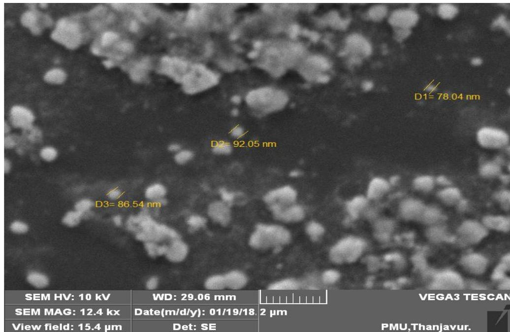
**Fig.3: SSEM image of synthesized AgNPs.**
