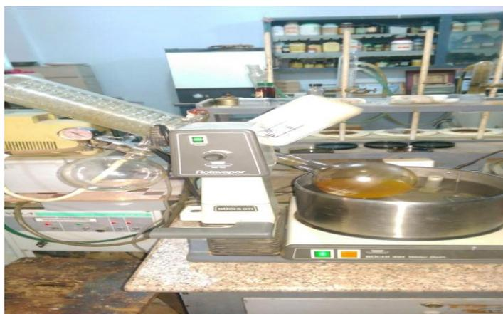
Fig. (1): Rotary Evaporator apparatus.
