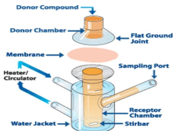
Figure 1: *In-vitro* diffusion cell fitted with Pig Skin.
