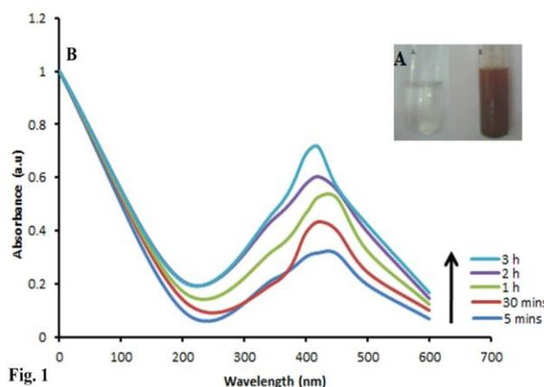
**Fig. 1.** (a) Aqueous solution of 10<sup>-3</sup> mM AgNO<sub>3</sub> with *Z. jujuba* seed extract (left) before adding the seed extract and (right) after addition of seed extract at 30 min. (b) UV-vis spectra of aqueous AgNO<sub>3</sub> with *Z. jujuba* seed extract at different time intervals.
