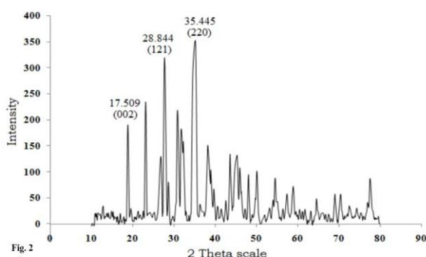
**Fig. 2.** XRD pattern of synthesized Ag NPs from aqueous seed extracts of *Z. jujuba*.
