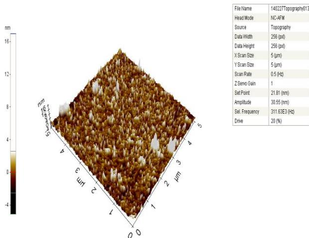
Fig. 5. AFM images of the synthesized Ag NPs showing (A) increased surface view and (B) 3D view
