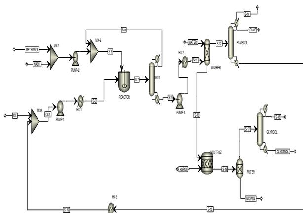
Figure. 1: Aspen Plus model of biodiesel process.
