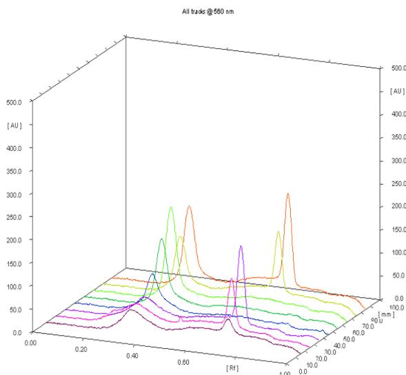
**Fig: Densitogram of standard and combination tablet of AM and LS in different concentrations at 560 nm.**
