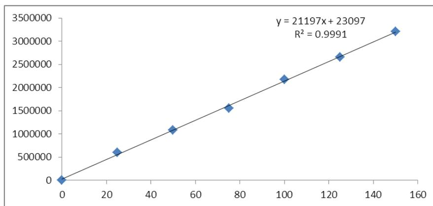
Fig 4: The linearity curve of Acalabrutinib concentration vs peak area.
