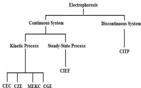
**Figure 1.3: Categorization of Electrophoresis Techniques.**
