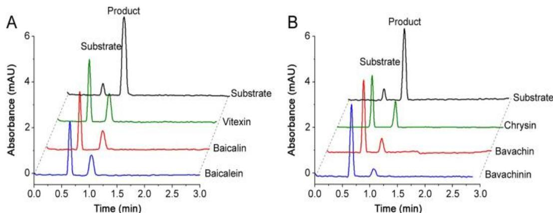
**Fig.4: Overlaid electropherograms for neuraminidase inhibitor screening by on-line immobilized enzyme assay detected at 320 nm with reference wavelength of 260 nm (A) and at 320 nm without reference wavelength (B).**
