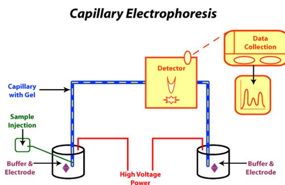
Figure: 1 Capillary electrophoresis setup.
