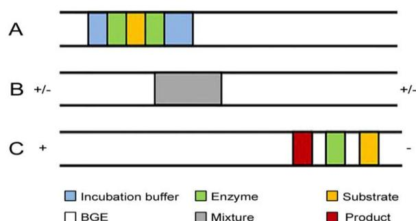
**Fig.3: Schematic overview of EMMA. (A) Sequential injection of the incubation buffer, tyrosinase, L-DOPA, tyrosinase, incubation buffer, BGE. (B) Mixing by applying a voltage switch sequence. (C) Mixture separation and product detection.**
